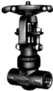
OS&Y gates. Threaded and socket weld ends 800 psi 850 degrees F. welded bonnet.
