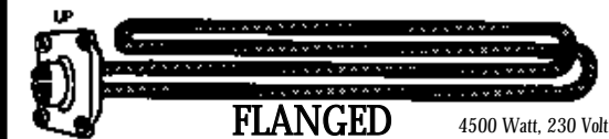
Lime-Life Elements - Highest grade nickel and chromium incaloy, ultra low-watt density, heats in lime and build-ups that will burn out ordinary elements. Best where water has high mineral content.
