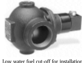
Low water fuel cut-off for installation in 2 1/2" tapping provided on some hot water boilers. Model 764.
