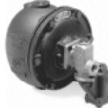
Make-up water feeder, for low pressure steam boilers, float operated, integral strainer monel seat, maximum water supply pressure 100psig maximum boiler pressure 25 psig. Model 25A.
