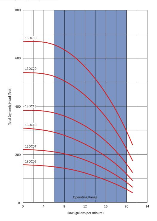
These curves are based on factory tests when pumping clear, fresh, non-aerated water at a temperature not exceeding 85°F. Due to production tolerances, these curves can vary plus or minus five percent.
