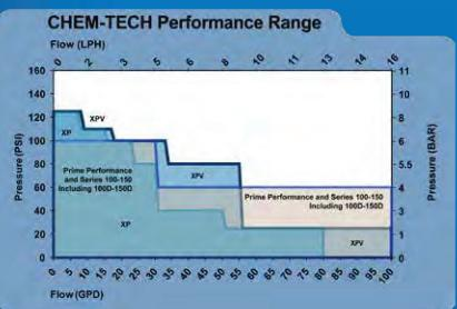
All Chem-Techs are tested and rated under hot conditions guaranteeing that the flow and pressure ratings meet the specifications.
