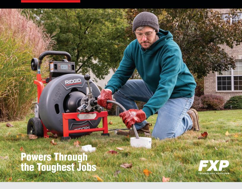
The RIDGID® K-4310 FXP™ Drum Machine is RIDGID's most powerful drum machine, delivering bestin-class performance. Powered by the FXP Technology platform, this battery-powered tool provides cordless freedom and powerful performance. The Cable Counter gives real-time feedback measuring cable distance in 3" to 10" lines on residential and commercial jobs, making this a valuable addition to your truck.
