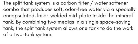
This split tank system provides for both activated carbon in the top chamber to remove chlorine and high-capacity softening resin in the bottom. This creates softened
