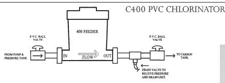
Non electrical chemical feed system. Powered by water pressure and operates only water is used. The C400 uses chlorine pellets and does require a carbon tank. U1 adapters up to  $1 \frac{1}{2}$ ".
